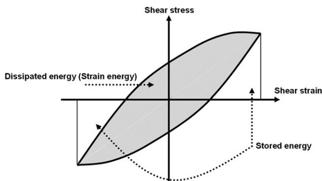
**Figure 1** A typical hysteresis shear stress–strain loop (Green, 2001).
